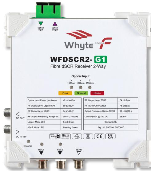
The optical dSCR multiswitch range from Whyte provides access to Sky Q, Legacy, TV and Radio services. The dedicated TERR Output can be amplified and/or split to provide additional TERR sources to bedrooms. Designed for use with the Whyte Fibre Optic product range these are typically used as home terminal units within a fibre to the home (FTTH) IRS system.
